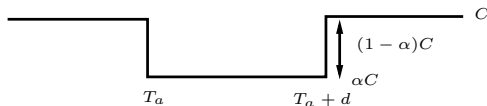
Figure: Depiction of the capacity profile under a weather-front based uncertainty set for a single affected airspace element.
